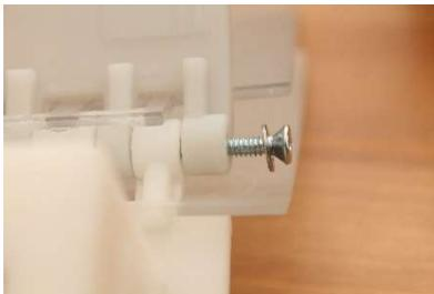
Add the screw between both links using a screwdriver and have a washer and bolt ready to the other side
